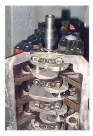
You then need to start with a Twin Cam engine, or at least everything above and in front of the block, and graft it all onto the MGB block. This sounds much easier than it turned out to be.
