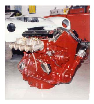
It would be possible to do a street conversion using original SU carbs and a 10:1 compression ratio to run pump premium gas, that would produce around 125 BHP in 1800 cc. form or 135 – 140 BHP in 1950 cc. form, but as most of these engines see only infrequent street use and rarely are run above 5000 RPM anyway, it would seem to me that this would be spending many thousands of dollars for mere bragging rights.
